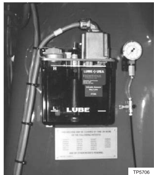
Figure 10.1 - Lube Unit Mounted on Left Side of Machine (1 Qt Capacity)
