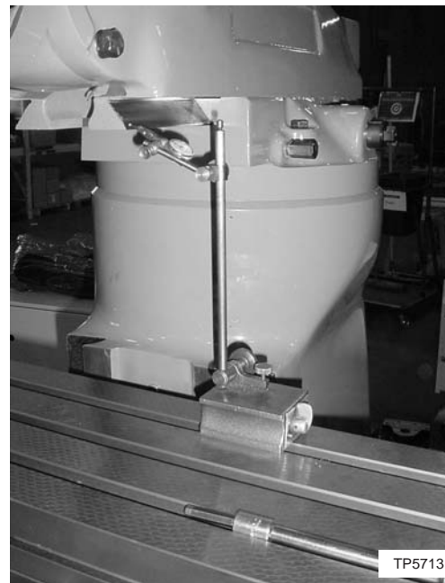
Figure 12.5 - Indicating off of Dovetail of Ram
